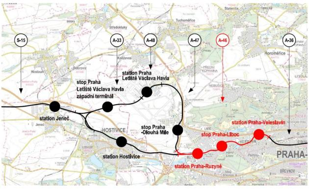
New stop Praha-Liboc will be built between Praha-Veleslavín and Praha-Ruzyně stations with two external platforms 220 m long and grade-separated access via an underpass.
