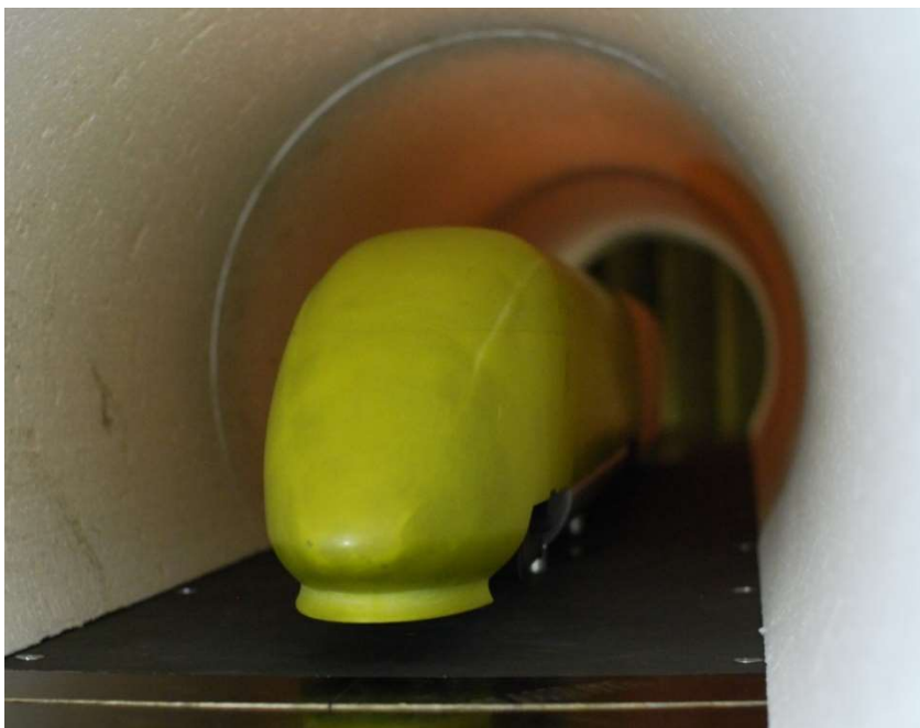
Obr. 2.4 Model ICE 3 v tubusu modelu tuneelu
