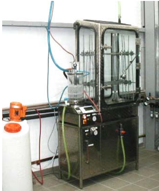
Figure 1: Photograph of the environmental ageing chamber HK400-BE used for salt mist and humid sulphurous atmosphere ageing for components used above ground
