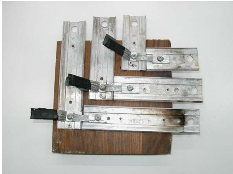
Figure 5: Photograph of specimens after environmental and electrical testing of 50kA (Class N)
