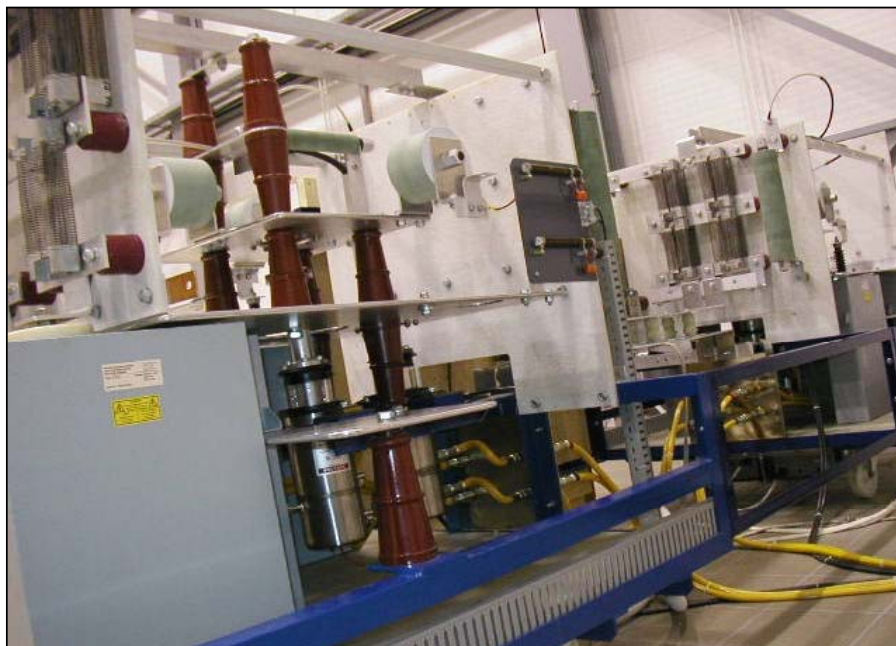
Figure 2: Photograph of the 100kA impulse current generator
